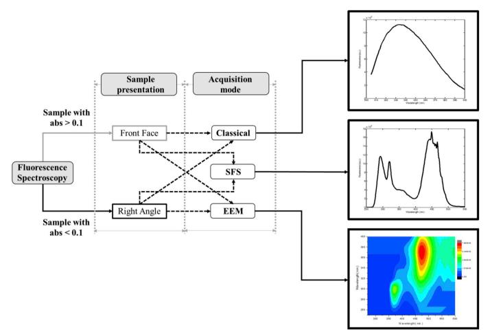
Fig. 3. Principal acquisition modes of fluorescence spectroscopy (see the text for the abbreviations).
